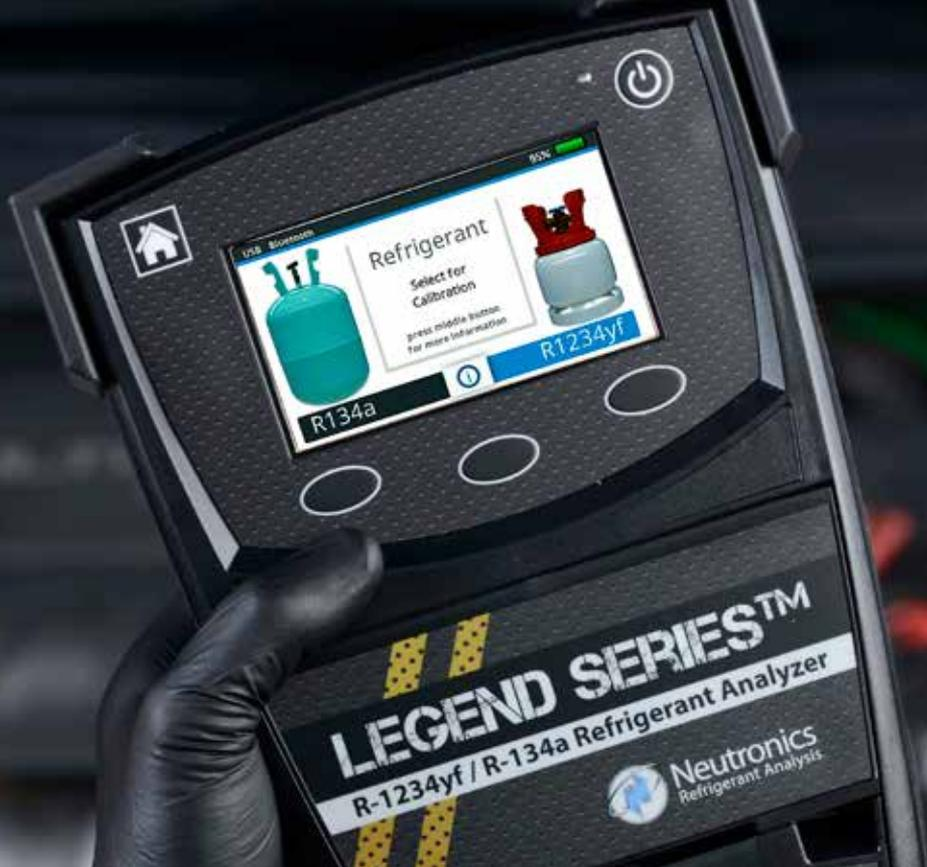
The award-winning Legend Series™ R-1234yf/R-134a Refrigerant Analyzer is equipped to service R-12, R-134a, and R-1234yf vehicles all in one tool. With advanced infrared technology this is a refrigerant analyzer for the past, present, and future.
