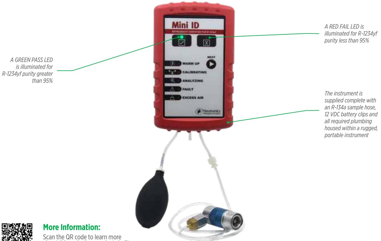
A GREEN PASS LED is illuminated for R-1234yf purity greater than 95%
